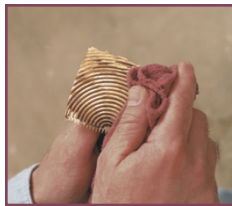
Note: Occasionally wipe off the face of the graining tool to prevent the grain pattern on the face of the tool from clogging.
